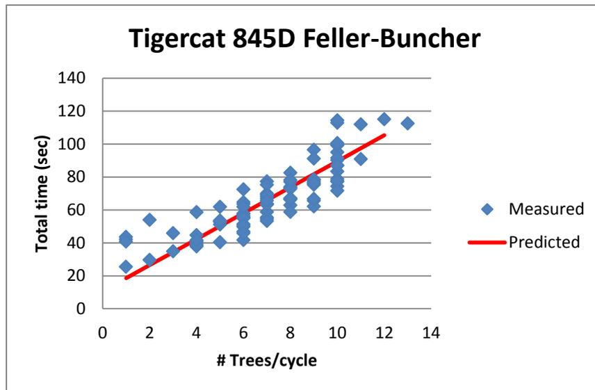
**Figure 1. Plot of time study data and regression equation for the feller-buncher.**
