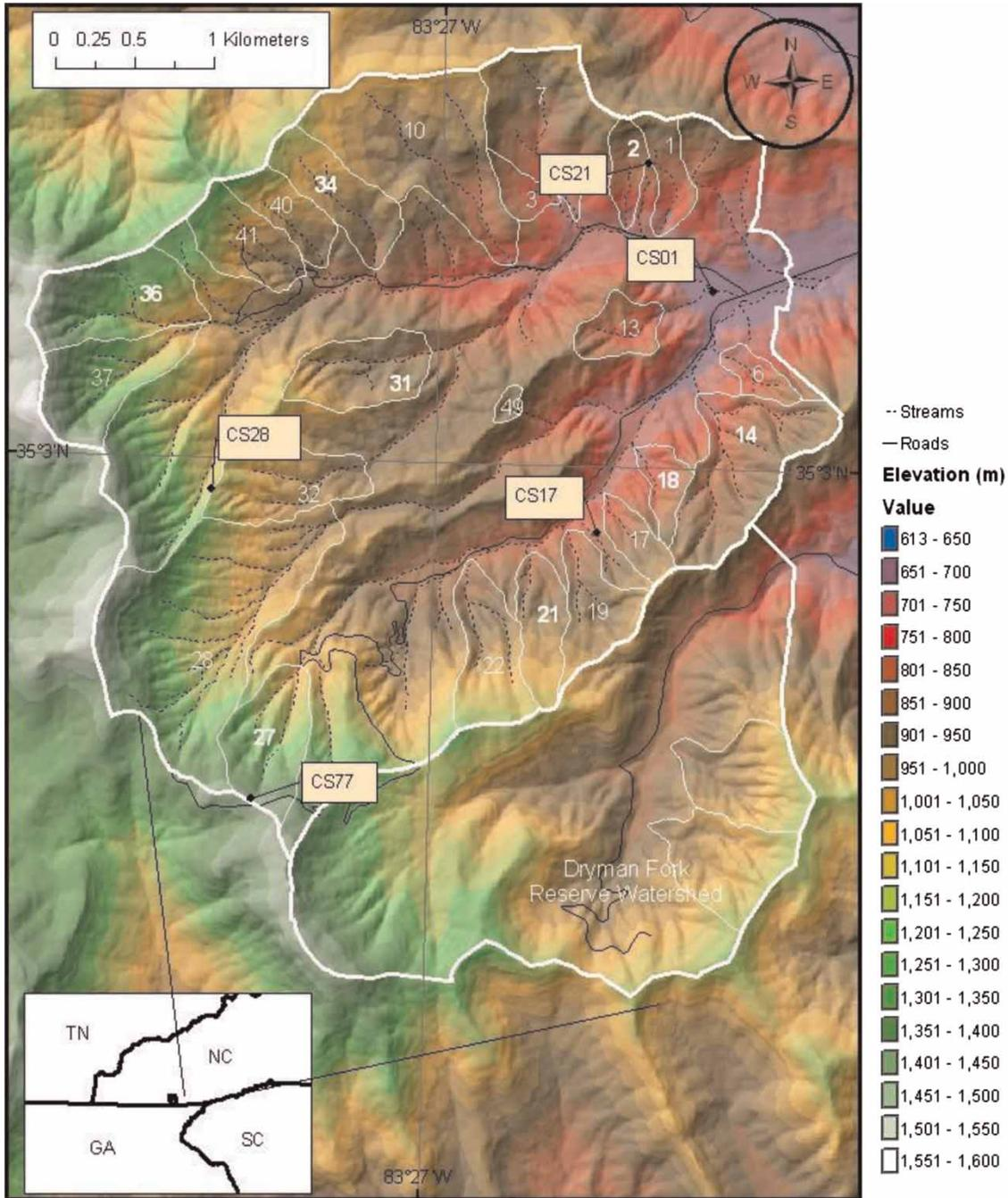
**Figure 1** | Elevation gradients and main and sub-watersheds (bold and non-bold white lines, respectively) at Coweeta Hydrologic Lab. Numbers denote reference (bold) and experimental (non-bold) watersheds. Climate stations are identified by white text. Inset: location of Coweeta Basin with respect to southeast USA.
