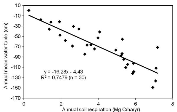
**Fig. 6** The relationship between annual soil CO<sub>2</sub> flux and annual mean water table on WS80
