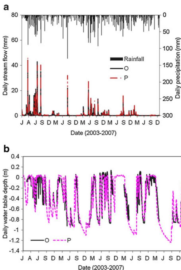
**Fig. 2** **a** Simulated and measured daily discharge in calibration period (2003–2004) and validation period (2005–2007). **b** Measured and simulated daily water table for an automatic well in calibration period (2003–2004) and validation period (2005–2007). *O* observation, *P* prediction
