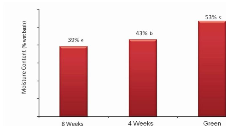
**Figure 2:** Moisture content of wood chips harvested fresh and allowed to dry four and eight weeks. Different letters indicate significantly different values ( $p < 0.05$ ).
