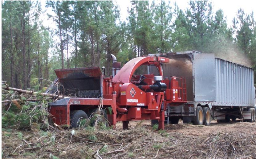
**Figure 1:** 600 horsepower Morbark 40/36 drum-style chipper.
