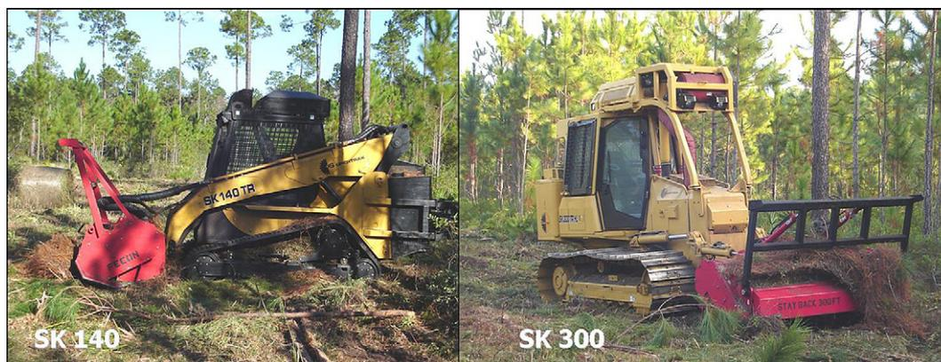
Fig. 2 – Supertrak tractors, SK 140 TR and SK 300 TR, with Fecon mulcher heads.
