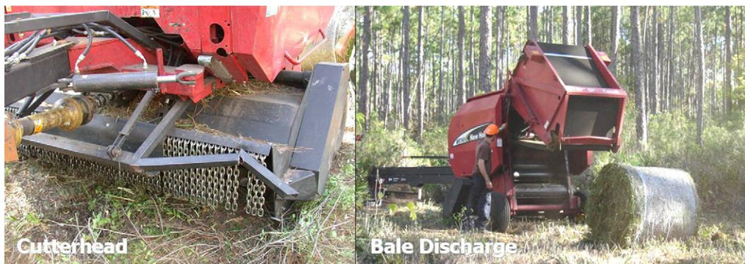
Fig. 1 – The Bio-baler operated by the Caterpillar Challenger MT565B tractor.
