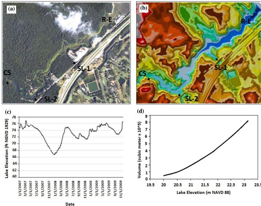
Figure 2. Reservoir-embayment (R-E) bathymetric data: (a) locations of cross-sections of the R-E, (b) LIDAR map of the R-E, (c) lake water levels for 2007–2009, and (d) volume versus lake elevation.
