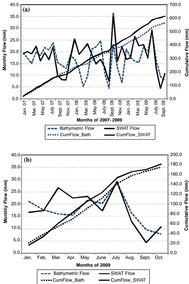
**Figure 7.** Bathymetric-estimated and SWAT-simulated monthly and cumulative monthly reservoir-embayment (R-E) outflow for (a) the 34-month (2007-2009) period and (b) ten months of 2009.
