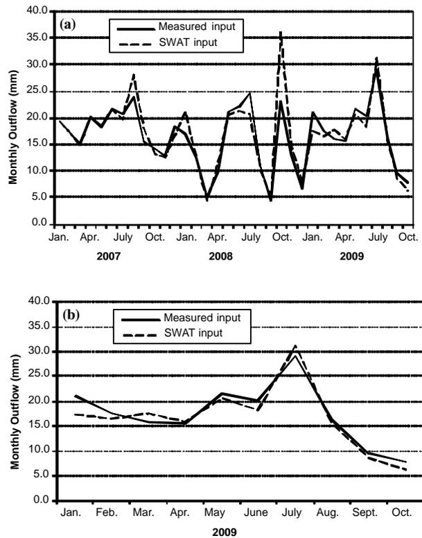
**Figure 9.** Estimated monthly R-E outflows for (a) the 34-month period using measured (solid line) and SWAT estimated (broken line) data and (b) the ten-month period in 2009 when data for all three stations were available.
