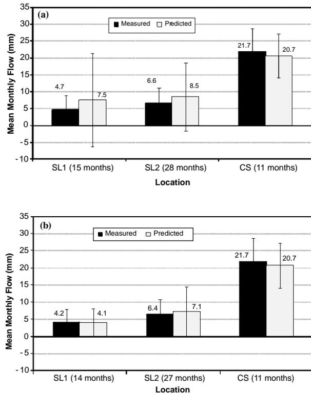
Figure 4. Measured and predicted mean monthly flows for SL1, SL2, and CS (a) with all data included and (b) with exclusion of October 2008 data with high flow events.
