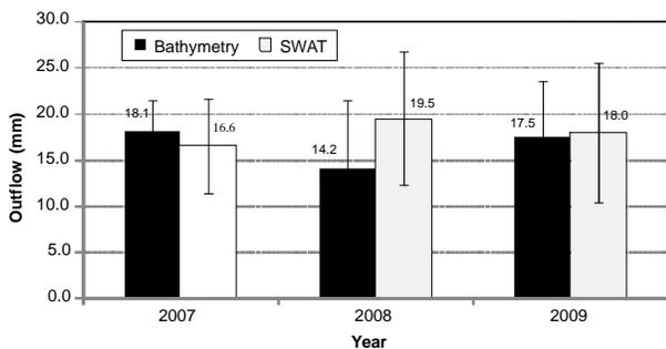
**Figure 8.** Measured (bathymetry) and SWAT-predicted mean monthly outflow from the reservoir-embayment (R-E) for each of the three years (2007-2009). Vertical bars are standard deviations.
