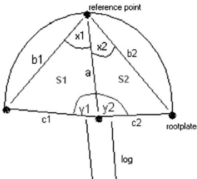
**Fig. 1** Measurement of pit area. Distances  $a$ ,  $b1$  and  $b2$ , and angles  $x1$  and  $x2$  from the reference point were recorded. Distances  $c$  and angles  $y$  can be derived using the sine and cosine theorems. Sections  $S1$  and  $S2$  were determined separately by calculating the disk sections of each and taking the average of  $c1$  and  $a$  as the radius of section  $S1$  and the average of  $c2$  and  $a$  as the radius of section  $S2$
