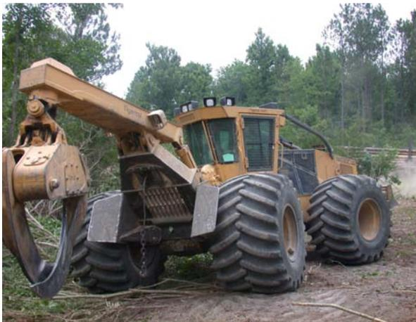
*Fig. 2: Additional equipment lights are common on extended shift operations.*
