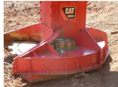
Figure 3: Data acquisition system for the dynamic temperature measurements mounted on felling head.
