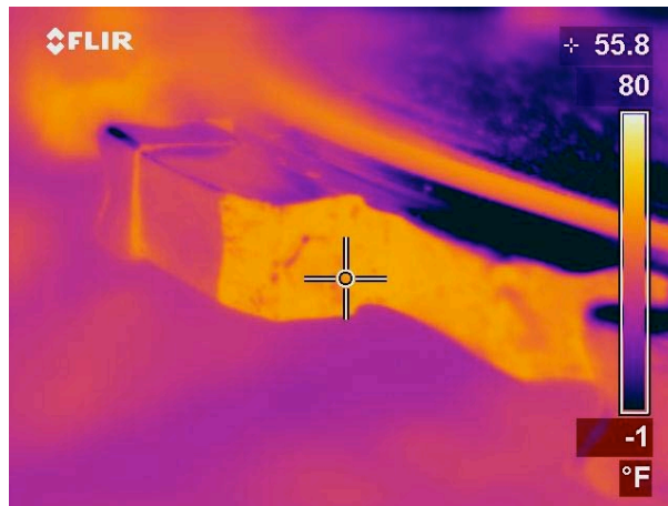
Figure 7: Infrared image showing temperature variation on the felling head.
