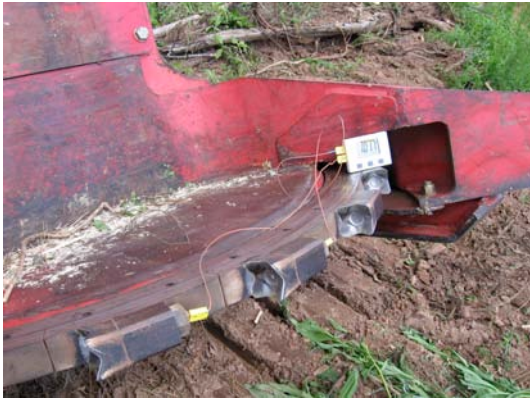
Figure 2: Modified bolts with thermocouples in place.
