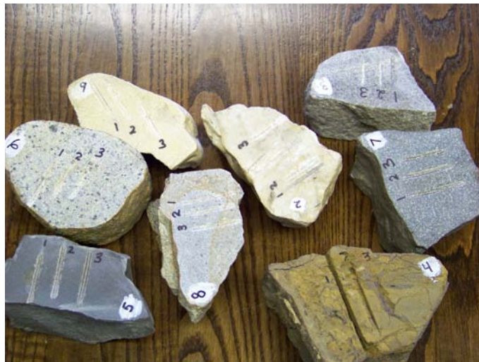
Figure 6: Rocks used in the sparking test, post testing.
