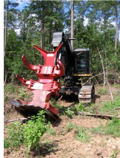
Figure 1: An example of a typical hotsaw felling head mounted on a tracked carrier.
