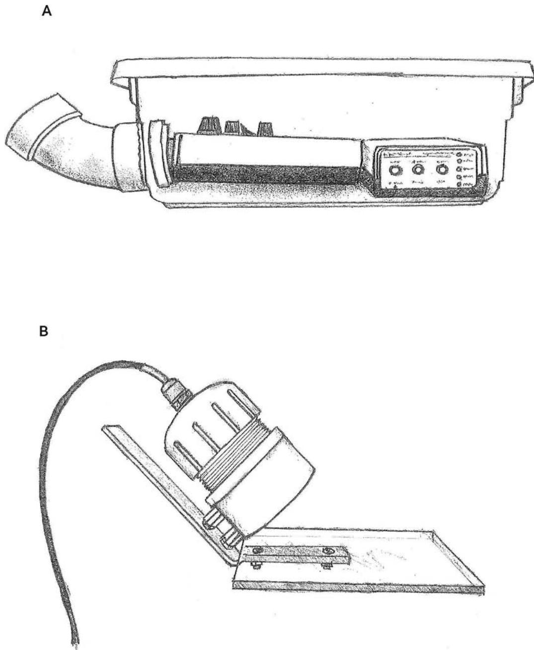
**Figure 1.** Schematics for the two weatherproofing options tested in this study. (A) the PVC weatherproofing option, and (B) the BatHat weatherproofing option. Both views are lateral views.
