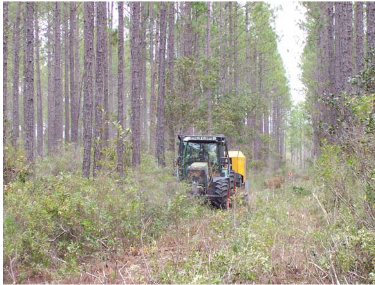
Figure 2. Baler making a second pass within a thinned row.
