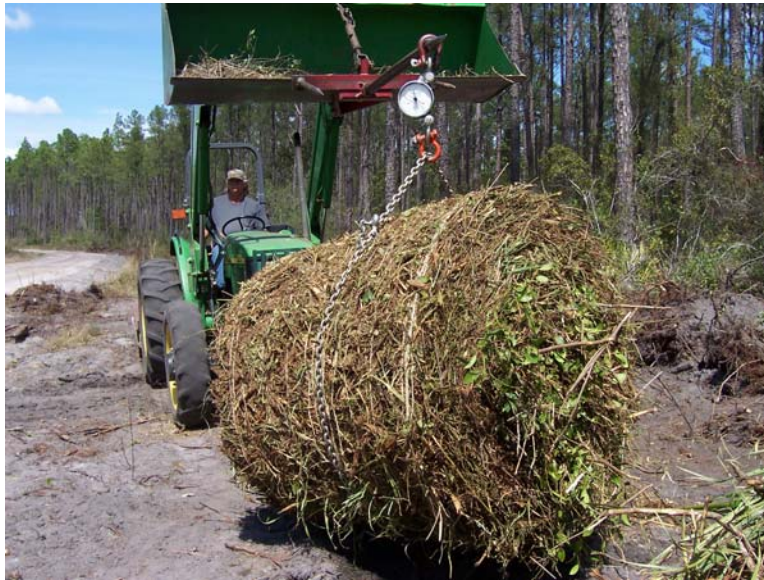
Figure 3. Obtaining green weight of a bale using a hanging scale.
