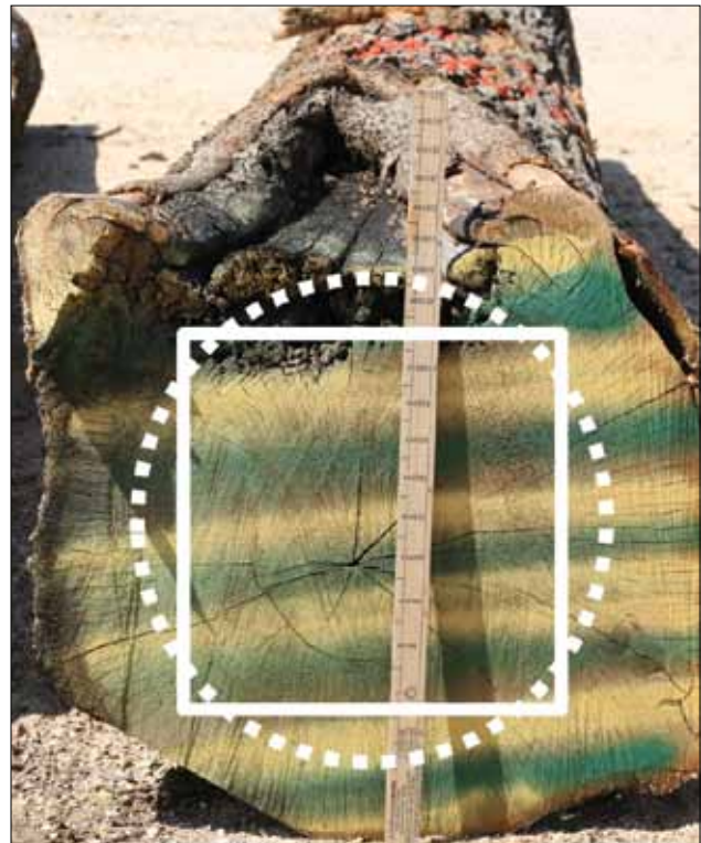
Figure 1—Fire scarred tree pre- and post-harvest. Tree DBH=19.7 inches, fire scar height=27.0 inches, fire scar depth=5.0 inches. The dotted circle on the base of the log depicts (to scale) the log's small end diameter; the solid square represents the portion of the round log that is utilized when manufacturing rectangular dimensional lumber. Though this tree appeared heavily defected while standing, it only experienced 8.0 percent value loss and 2.8 percent volume loss, with much of the fire-caused defect removed during the milling process.
