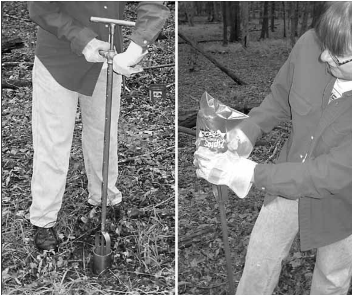
Figure 1—Using the single root auger to collect soil charcoal in Great Smoky Mountains National Park. The photo on the right shows the extrusion of a 10-cm core increment into a labeled plastic bag. (Photos by Matthew Valente)
