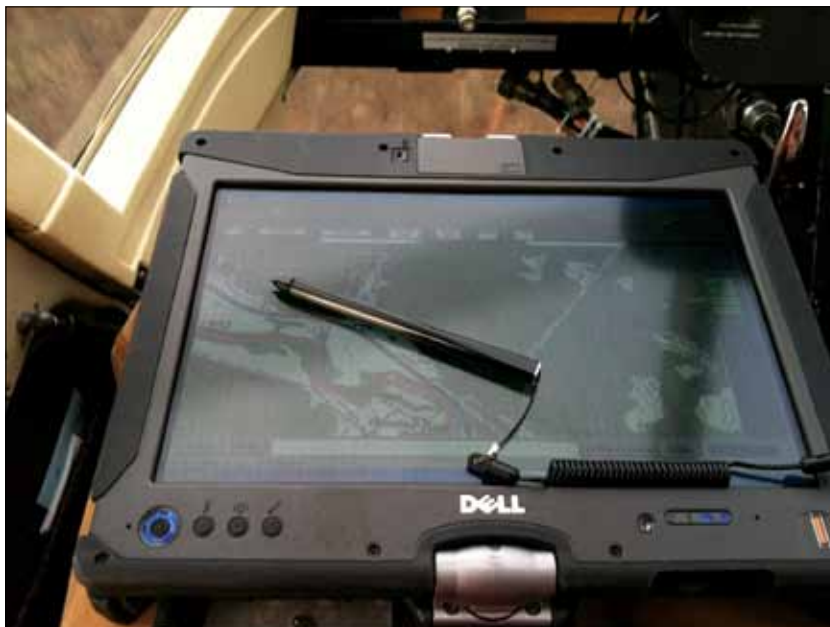
Figure 2—Digital sketch mapping software tablet used to survey female Ailanthus during helicopter surveys.
