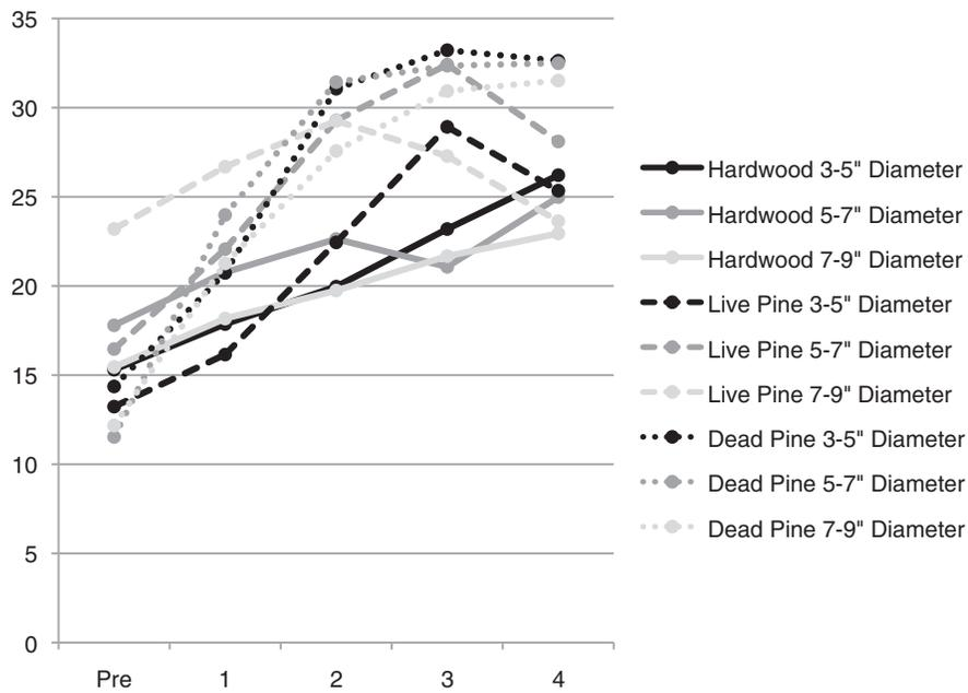
Figure 3—Average log moisture content (percent) prior to treatment (pre) and 24 hours after each rainfall event (1, 2, 3) for the treatment of 1 inch of rain applied four times over a 1-week period.
