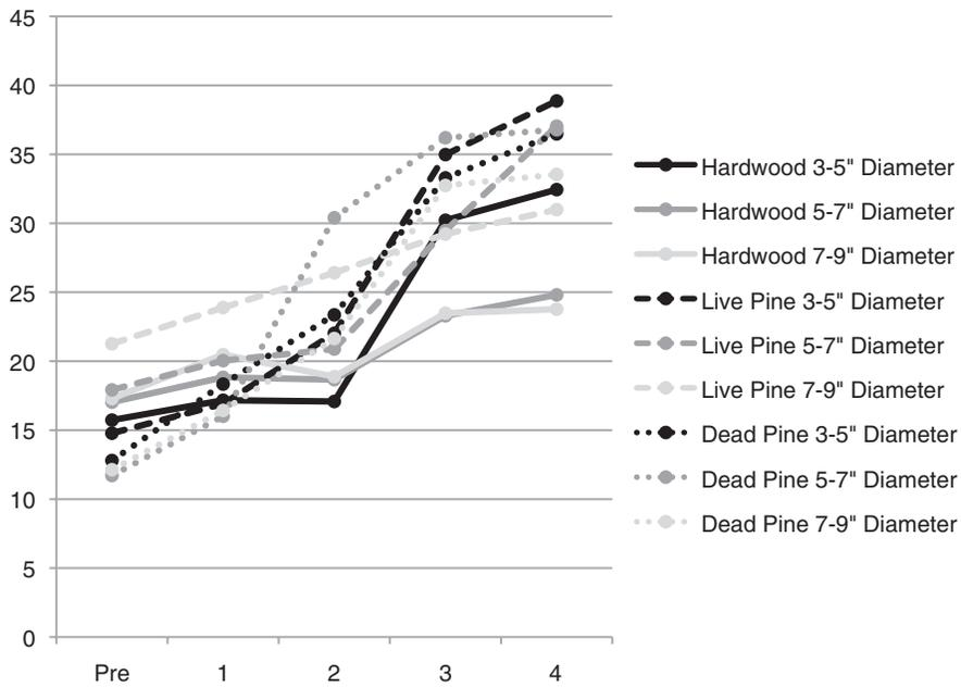
Figure 5—Average log moisture content (percent) prior to treatment (pre) and 24 hours after each rainfall event (1, 2, 3, 4) for the treatment of 1 inch of rain applied four times over 2 weeks.
