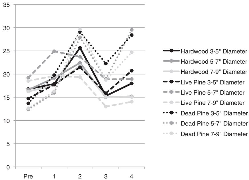
Figure 7—Average log moisture content (percent) prior to treatment (pre) and 24 hours after each rainfall event (1, 2, 3, 4) for the treatment of 1 inch of rain applied four times over 4 weeks.
