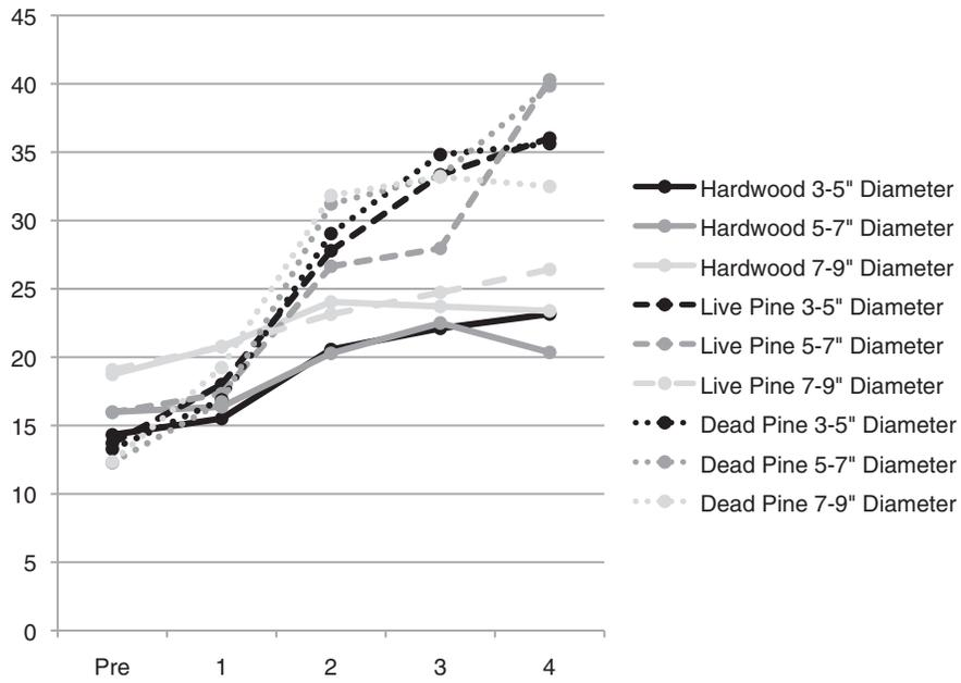
Figure 6—Average log moisture content (percent) prior to treatment (pre) and 24 hours after each rainfall event (1, 2, 3) for the treatment of 1 inch of rain applied four times over 3 weeks.
