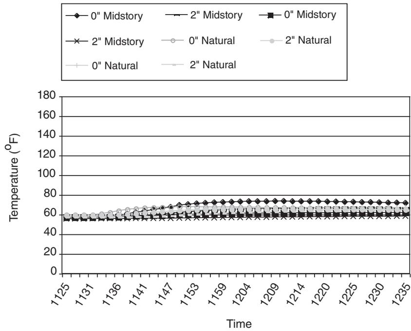
Figure 1—Temperatures (°F) in the block treated with Tim-bor® during a spring burn from probes at 0 and 2 inches below the duff in a plot with added midstory fuel and an adjacent natural fuel plot.
