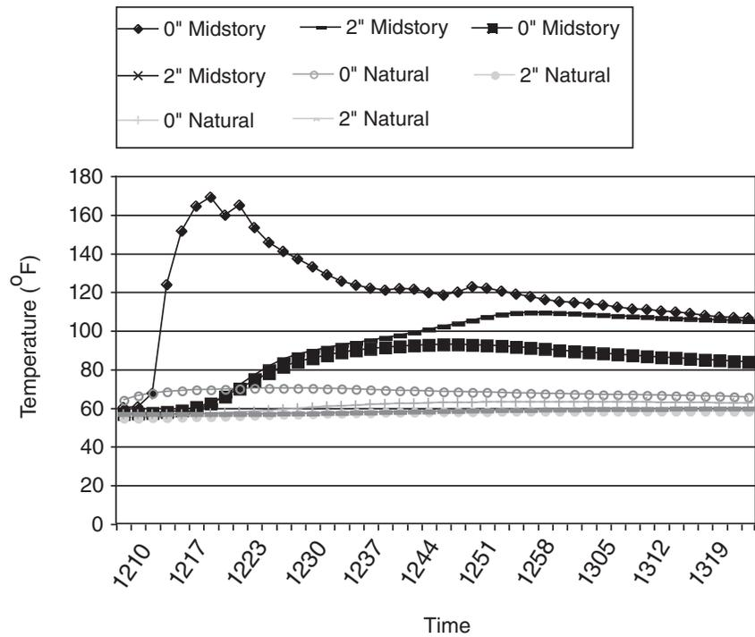
Figure 2—Temperatures (°F) in the No Stump Treatment block during the burn from probes at 0 and 2 inches below the duff in a plot with added midstory fuel and in an adjacent natural fuel plot.
