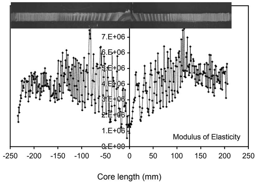
Figure 2—Modulus of Elasticity variation across an increment core.
