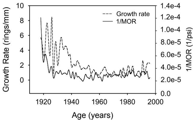
Figure 3—Variation of 1/Modulus of Rupture and growth by year.
