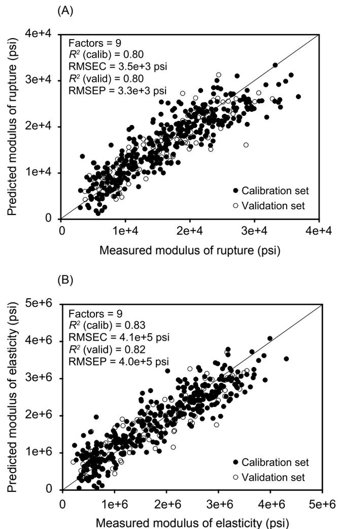
Figure 1—Relationship between predicted and measured (A) Modulus of Rupture and (B) Modulus of Elasticity.
