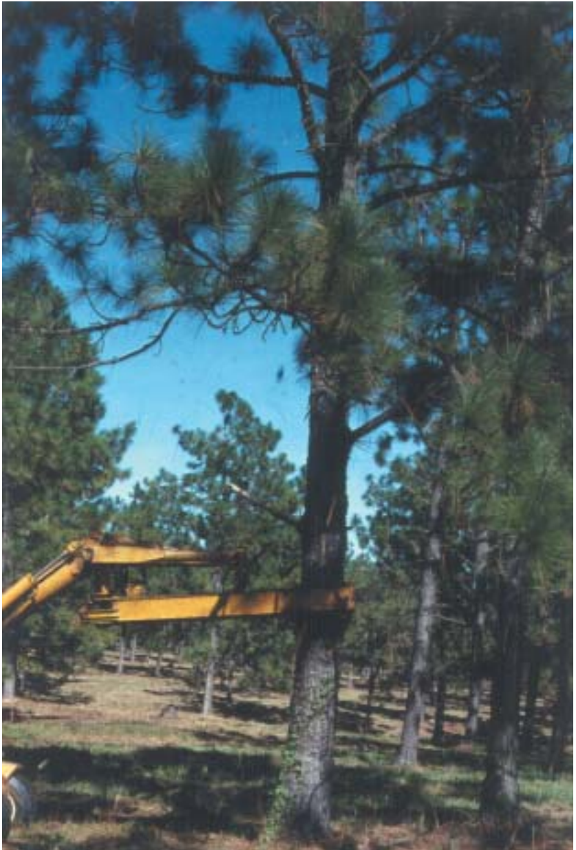
Figure 5—Collecting longleaf pine cones in a seed orchard with a cone shaker.
