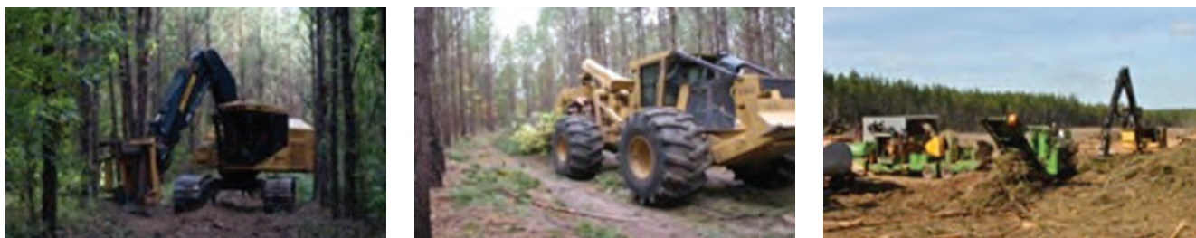
Figure 3.6 | Machines for harvesting trees and forest residues
