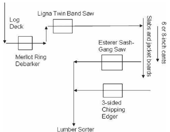
Figure 5. — Schematic diagram of sawing sequence.
