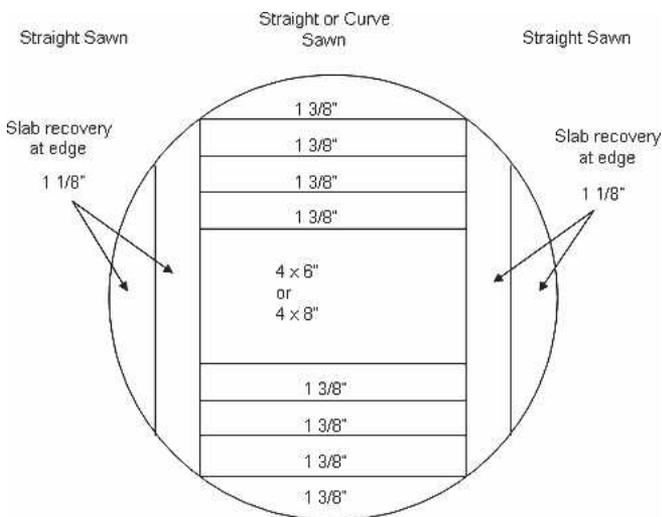
Figure 6. — Diagram of sawing pattern used to saw logs for both straight and curve sawing log groups.
