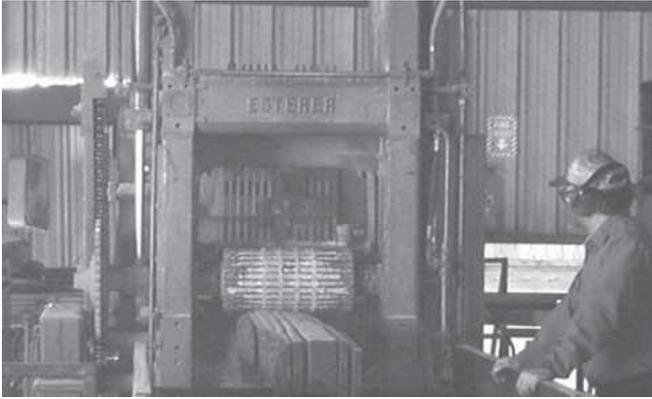
Figure 1. — Photograph of Esterer sash gang saw. This saw was used to both curve saw and straight saw the study logs from each sweep group.
