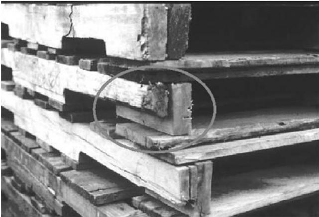
Figure 3. — Example of plug companion stringer repair.
