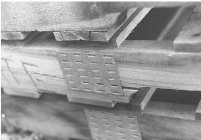
Figure 4. — Example of metal plate stringer repairs.
