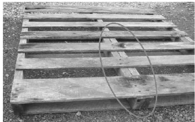
Figure 2. — Example of half companion stringer repair.
