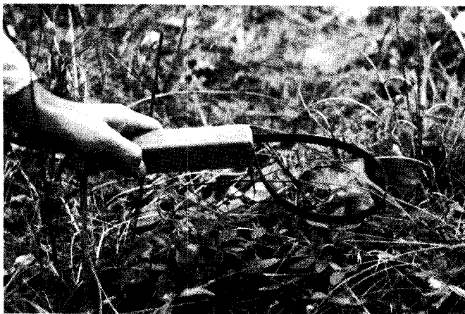
Figure 1 --Loop-densimeter used in estimating foliar cover.
