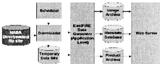
Figure 3. Data flow of the EastFIRE real time RS data processing system.
