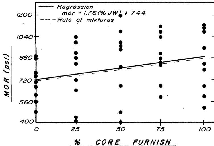
Figure 4. — Modulus of rupture after ODVPS exposure of 40-pcf fiberboard made from mixtures of juvenile (core) and mature southern pine furnish.
