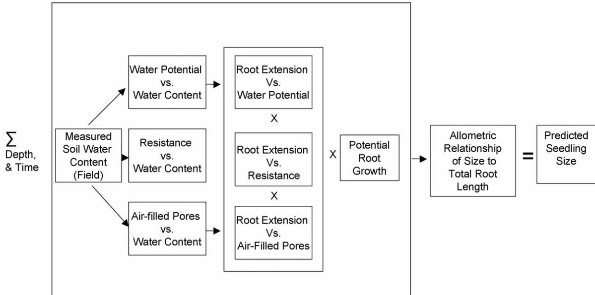
Fig. 1. Schematic diagram illustrating general structure of model predicting seedling growth. Soil water content is used to estimate soil water potential, mechanical resistance and air-filled pore space based on site-specific and generalized relationships. Root growth is reduced below potential growth (optimal) and converted to above-ground growth using an allometric relationship.
