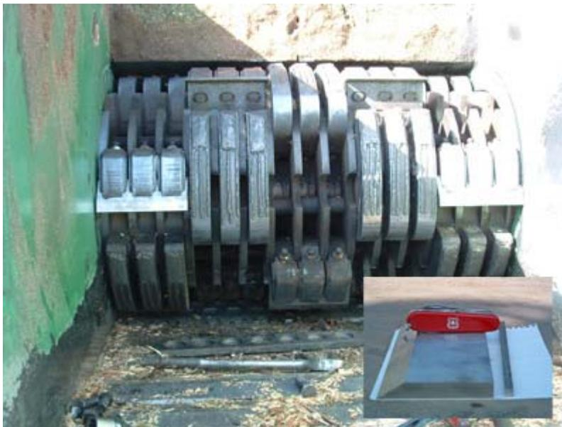
*Fig. 3: ProGrind H-3045 planer knives (inset shows scale).*
