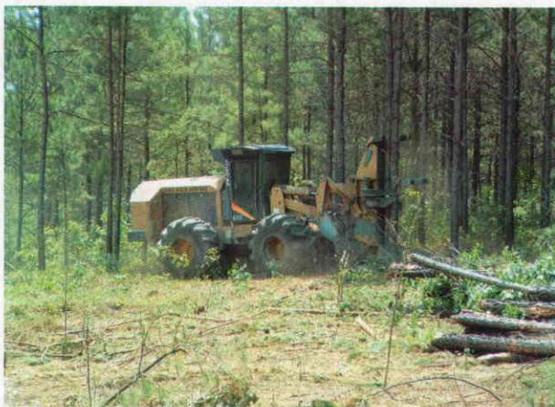
*Fig. 2: Hydro-Ax 670 feller-buncher at work.*
