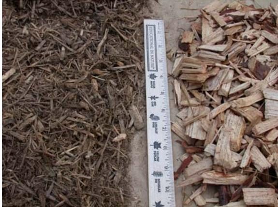
Figure 1. Re-ground whole-tree chips from tub grinder (left), whole-tree chips from chipper (right).
