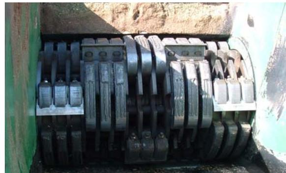
Figure 2. Modified ProGrind H-3045 drum
