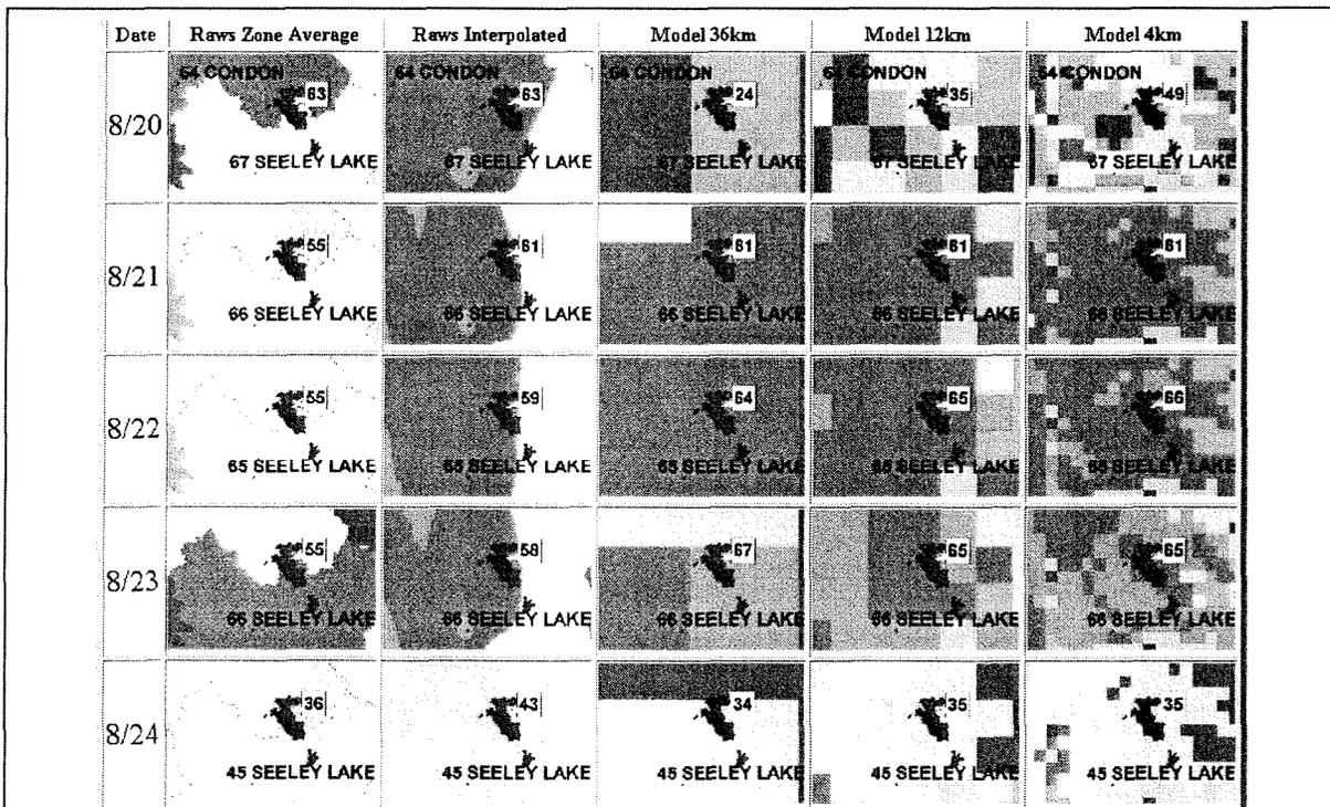
Fig. 2. Comparison of observed ERC with Model forecast ERC for the Monture Spread Ridge Complex, August 2000. The color scale ranges from green for low values through yellow to orange and red for high values. The Fire perimeter is shown in red.
