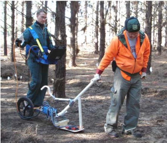
Figure 1. SIR 2000 Ground-penetrating radar system used with a forest survey rig, comprised of a high-frequency GPR antenna mounted on a stabilization board (1.5 GHz) and a survey wheel.
