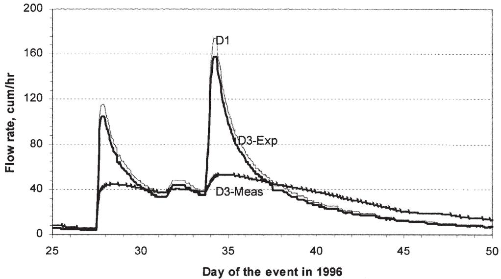
Figure 5. Comparison of hourly event hydrographs for expected (dark solid) and measured (light solid) with flow data from the watershed with orifice-weir treatment (D3) for the event of Day 27, 1996 at Carteret site. Data from watershed D1 (thin line) under conventional drainage is also presented.
