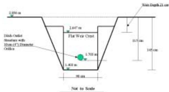
Figure 1. Schematic of a flat weir with an orifice hole installed on the riser structure at the ditch outlet of the watershed.
