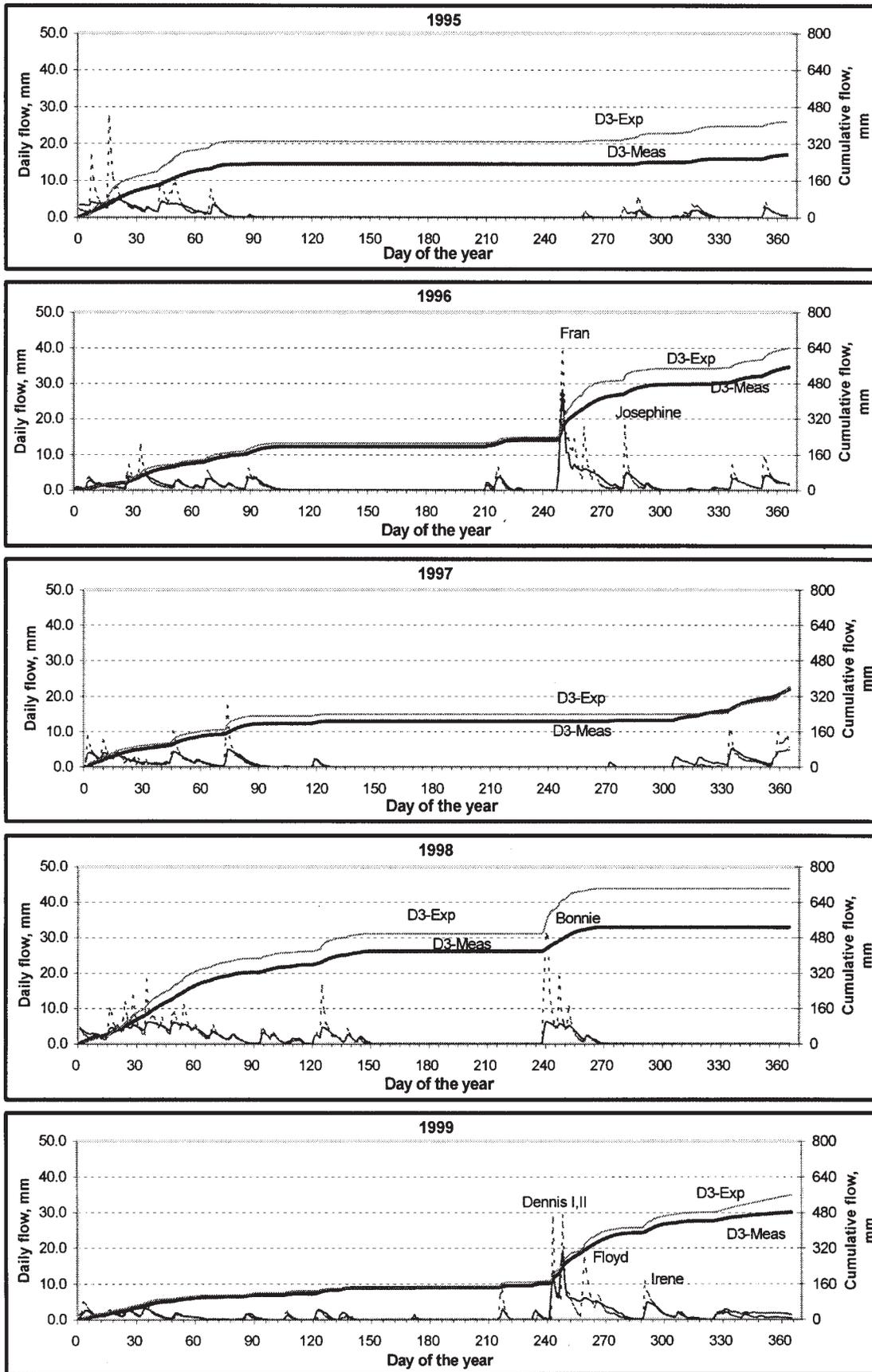
Figure 4. Measured (thick solid) and expected (thin dotted) daily flows and measured (thick solid) and expected (thin solid) daily cumulative outflows measured at watershed D3 with an orifice-weir treatment at Carteret site.
