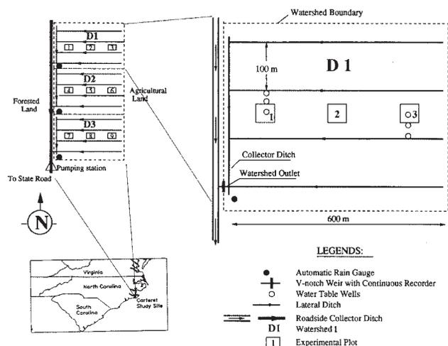
Figure 2. Schematic of the location and layout of the experimental watersheds D1, D2, and D3 at Carteret study site, North Carolina (after Amatya et al. 1998). D1 is the control with conventional drainage and D3 has an orifice-weir.
