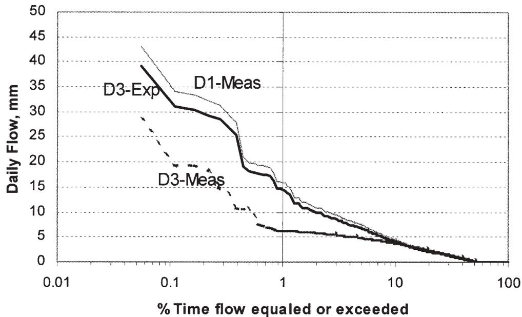
Figure 6. Comparison of daily flow duration for expected (thick solid) and measured (thick broken solid) flow data from the watershed with the orifice-weir treatment (D3) at Carteret site. Data from watershed D1 (thin solid) under conventional drainage is also shown.
