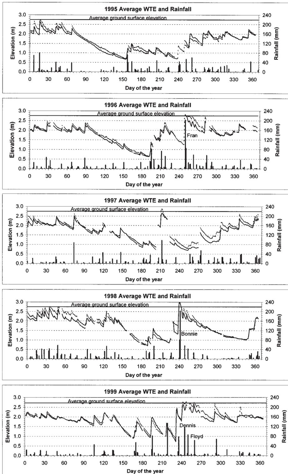
**Figure 3. Measured (dotted line) and expected (solid line) daily average water table elevations for watershed D3 with an orifice-weir treatment. Daily rainfall is also shown on secondary axis with solid bars.**
