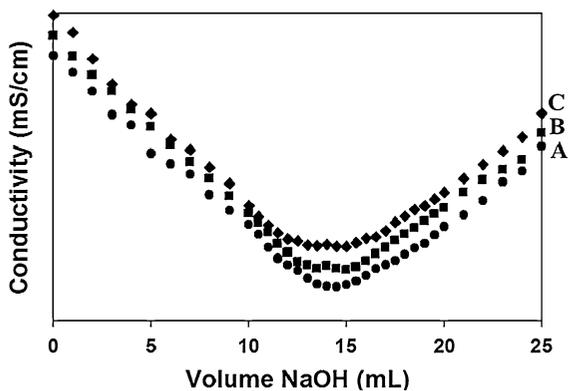
**Fig. 1** Conductimetric titration curves of TEMPO-mediated oxidized NFC with different DOs: non-oxidized (*Circle*), *A*, oxidized with DO = 0.1 (*Square*), *B*, oxidized with DO = 0.2 (*Diamond*), *C*
