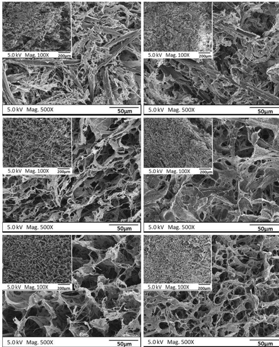
**Fig. 4** SEM of the aerogels based on NFC having different degree of oxidation without the addition of HAp (*Left*) and with the addition of HAp (*Right*). From the top to the bottom: DO = 0, 0.1, and 0.2
