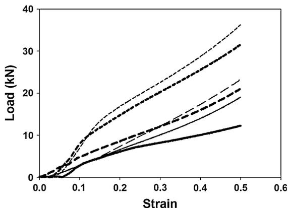
**Fig. 7** Rheological properties of the NFC-based aerogels. *Bold lines* represent the aerogels without HAp addition. *Solid line*: AG DO = 0; *long dashed line*: AG DO = 0.1; *short dashed line*: AG DO = 0.2
