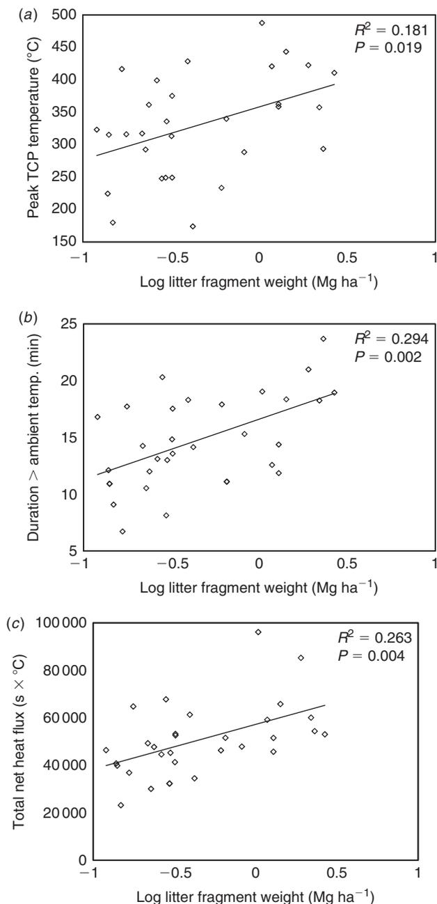
**Fig. 4.** Relationship between the weight of litter fragments and (a) peak thermocouple probe (TCP) temperature, (b) duration above ambient temperature and (c) total net heat flux during prescribed burns on longleaf pine xeric sandhill sites without duff.
