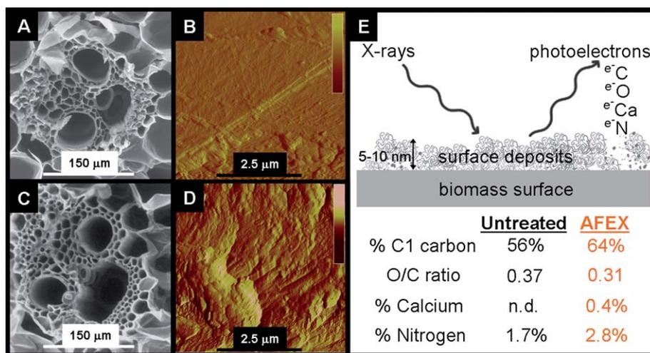
**Fig. 2** SEM and AFM amplitude images for untreated (A and B) and L-AFEX (C and D) treated corn stover. ESCA-based surface atomic composition (E) of untreated and L-AFEX treated corn stover. Color legend (dark-light shades) for AFM images depicts the amplitude current scale (0–2.5 volts). n.d. stands for 'not detected'.
