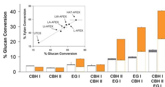
**Fig. 5** Glucan hydrolysis yield (24 h) of untreated (UTCS; left bar in grey) and L-AFEX treated corn stover (right bar in orange) by purified *Trichoderma reesei* cellulases. Empty and filled bars depict glucose and cellobiose yields, respectively. Inset depicts glucan and xylan hydrolysis yields (15 FPU Spezyme CP per g glucan loading) for corn stover treated with various AFEX severities.
