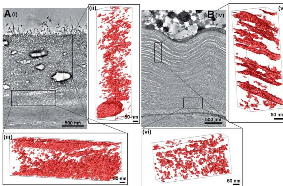
**Fig. 4** Modeling porous regions within HAT-AFEX (A: i–iii) and LW-AFEX (B: iv–vi) pretreated cell walls using 3D-TEM tomograms. Isosurface mesh enclosing pore spaces within a HAT-AFEX cell wall (i) sub-volume of S3 layer (ii) and S2 delamination zone (iii). Isosurface mesh enclosing pore spaces within a LW-AFEX cell wall (iv) sub-volume of the S2 layer (v) and S1 layer (vi).
