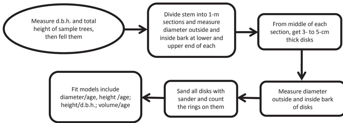
Figure 1--Details of field research and lab work.
