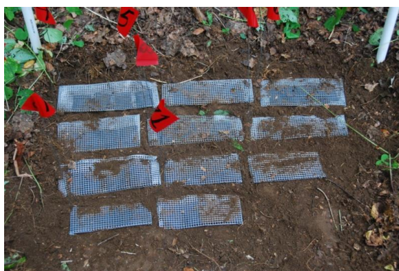
Figure 5--Bags enclosed in a wire mesh 'sandwich' and buried in contact with mineral soil. Bags are attached to flags to facilitate retrieval.
