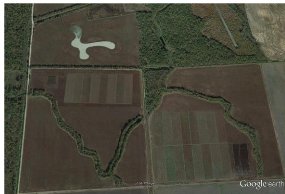
Figure 1--Google Earth™ imagery dated November 12, 2012 clearly delineates the physical layout of the 24 experimental units located in Washington County, MS on U.S. Army Corps of Engineers land situated near the eastern boundary of Leroy Percy State Park, the wooded area on the left edge of the picture. Each of the 24 units is 2.5 acres in size with rectangular dimensions of 660 feet long and 165 feet wide. The image (© 2013 Google Inc. All rights reserved) is centered approximately on the coordinates 33° 09' 11.81" N latitude 90° 54' 26.09" W longitude.
