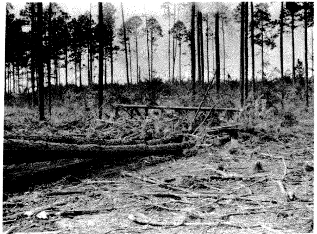
Figure 1.--A grapple skidder load being backed through a delimbing gate.
