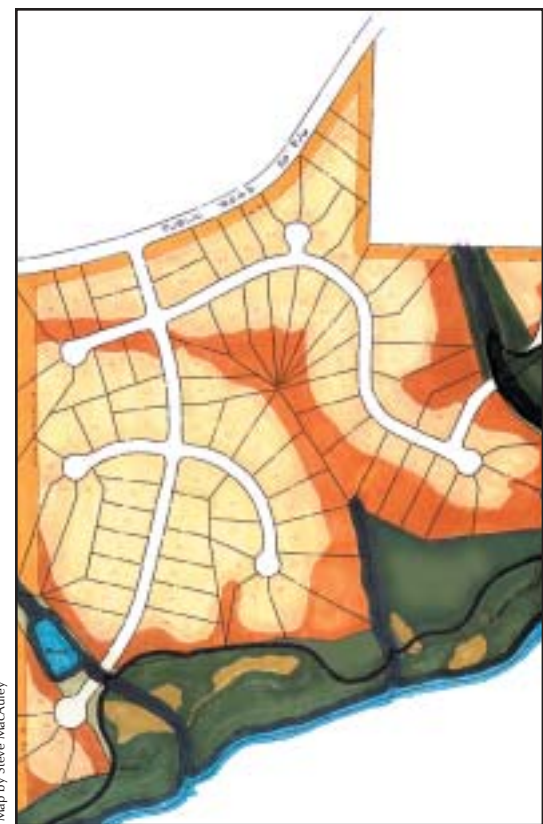
Figure 4.4 Alternative zoning techniques provide greater flexibility than traditional zoning and allow planners to design developments that better fit the land and to set aside more green space.
