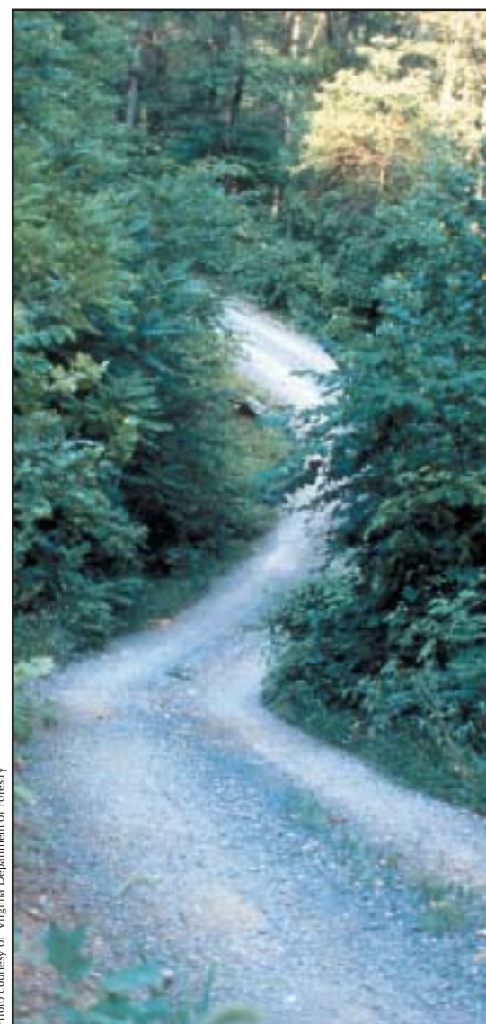
Figure 8.6 Steep, winding, narrow roads to residences may not be accessible by large fire engines or may become blocked with debris during a wildland fire.
